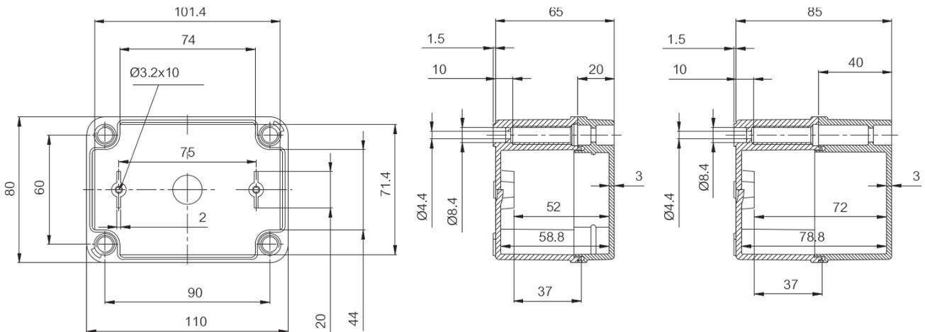
Illustration 4: Housing dimensions (in mm). Note: Drawing not including the cable gland.
