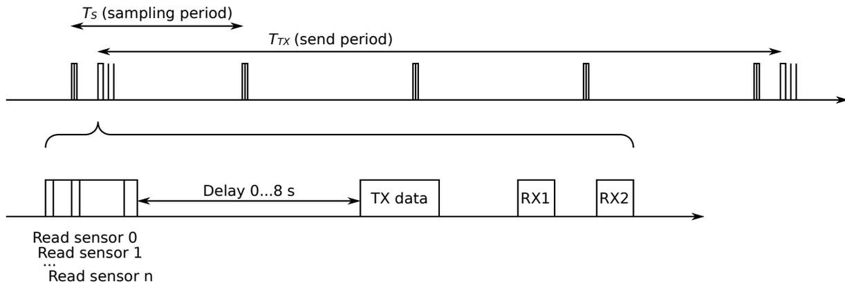
*Illustration 3: Device activity during the active mode. Shown in this diagram:  $T_{TX} = 4 \cdot T_S$ ; default for DL-LP8P:  $T_{TX} = 10 \cdot T_S = 10 \text{ min}$ .*
