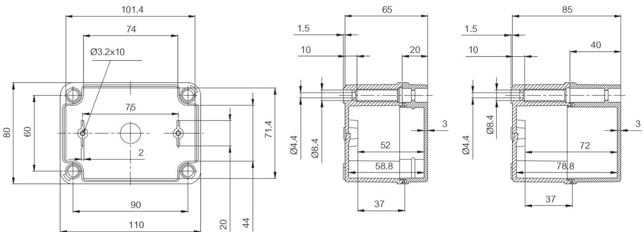
Illustration 4: Housing dimensions. Note: Drawing not including air inlet. Dimensions in mm.
